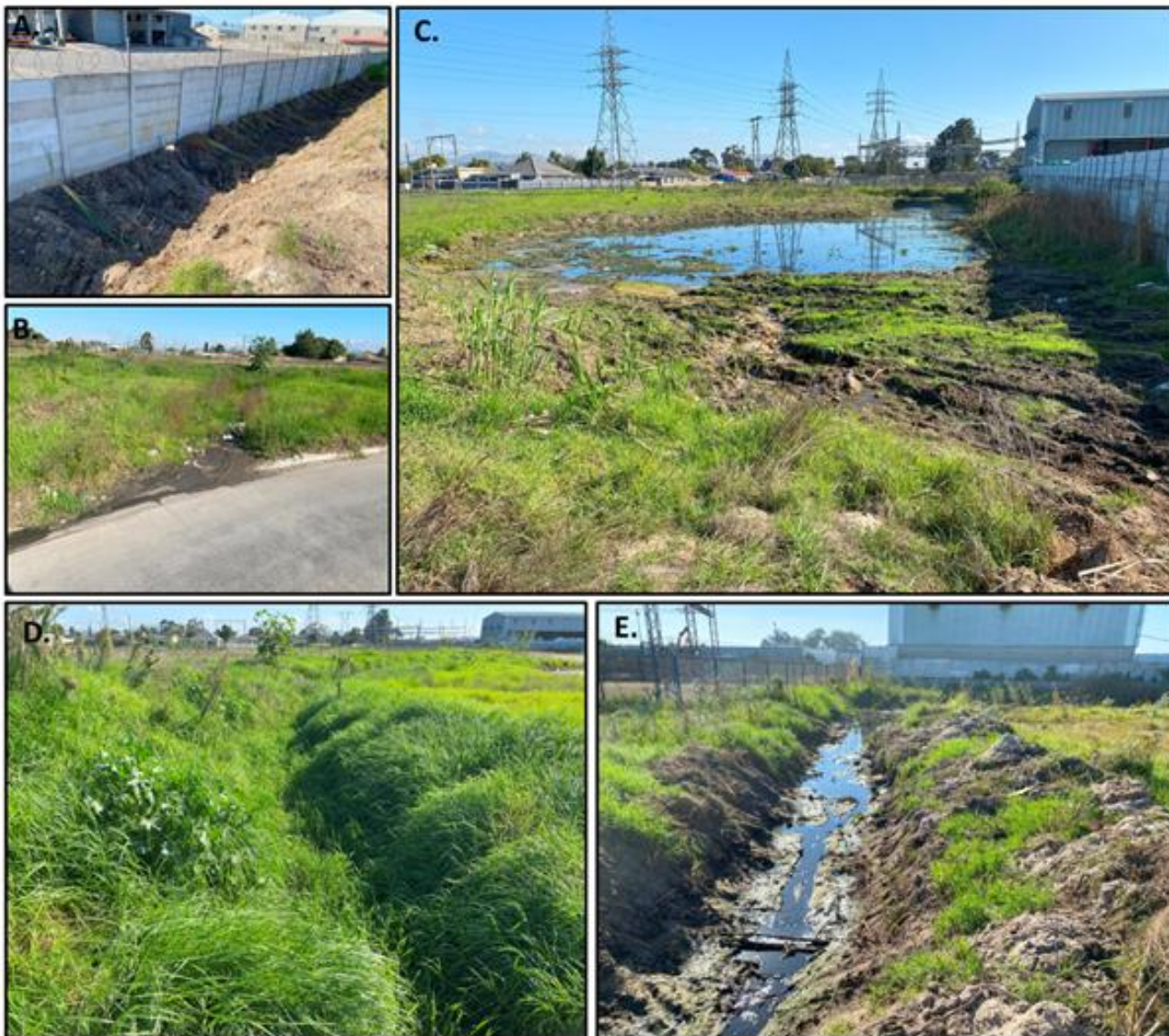
Figure 8. Photographs of the wetland on Erf 21593, showing, (A) the locations where run-off from Erf 21596 enters the wetland; (B) the location where run-off from the roads of the Kraaifontein industrial area flows into the wetland; (C) the permanently inundated wetland area against the boundary wall of the site ;(D) the channel of the wetland flowing from the east; and (E) the channel flowing to the west around erf 10268.
